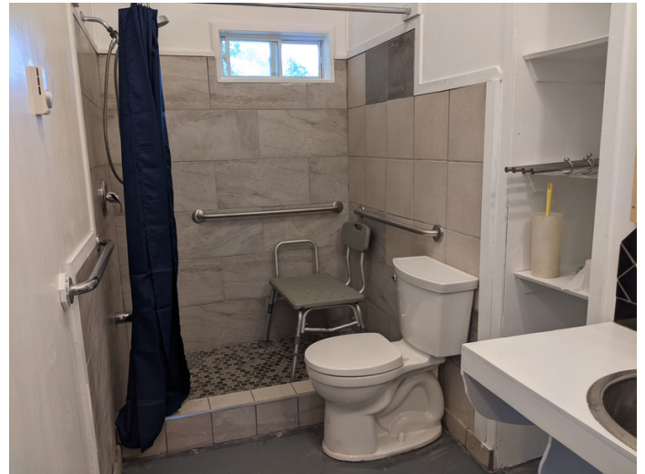
Dave's B washroom has a low step to get into the shower, a wide shower seat and grab bars
